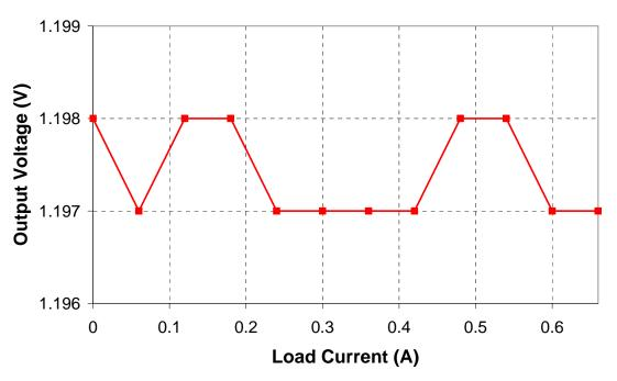
1.2V@0.66A Output Voltage vs. Load Current
