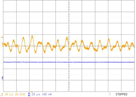
Fig 20: Output Ripple 3.3V (Ch1) @ 0.165 (Ch4) TPS 62200 DCDC, Low Line 3.6Vin, converter in PWM mode
