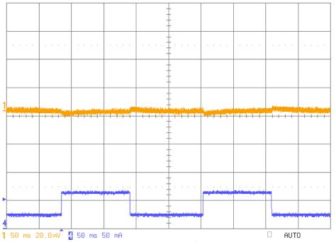
Fig 5: Load transient response on TPS71701, 1.2V output (Ch1) for load step 20mA to 60mA (Ch4 -33% to 100%), at high line 6Vin
