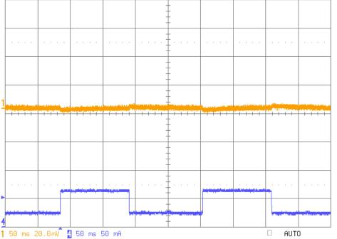
Fig 4: Load transient response on TPS71701, 1.2V output (Ch1) for load step 20mA to 60mA (Ch4 -33% to 100%), at low line 3.6Vin
