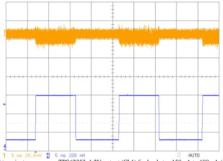
Fig 12: Load transient response on TPS62353, 1.2V output (Ch1) for load step 150mA to 600mA (Ch4 - 25% to 100%), at high line 6Vin
