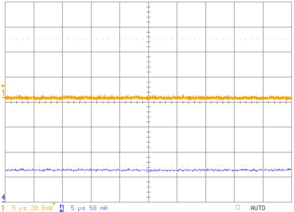
Fig 3: Output Ripple 1.2V @ 0.06A TPS 71701 LDO, 5Vin
