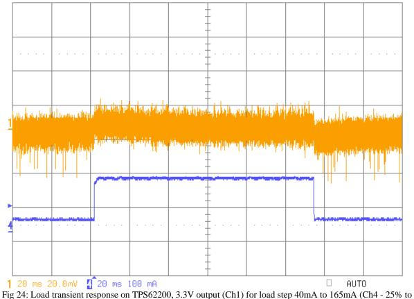
Fig 24: Load transient response on TPS62200, 3.3V output (Ch1) for load step 40mA to 165mA (Ch4 - 25% to 100%), at high line 3.6Vin
