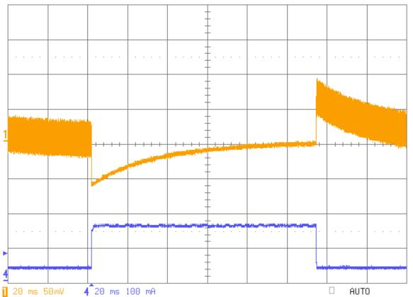
Fig 22: Load transient response on TPS62200, 3.3V output (Ch1) for load step 40mA to 165mA (Ch4 - 25% to 100%), at high line 6Vin
