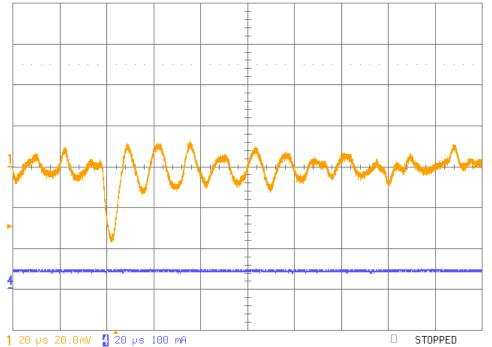
Fig 21: Output Ripple 3.3V (Ch1) @ 0.04 (Ch4) TPS 62200 DCDC, Low Line 3.6Vin, converter in PFM mode
