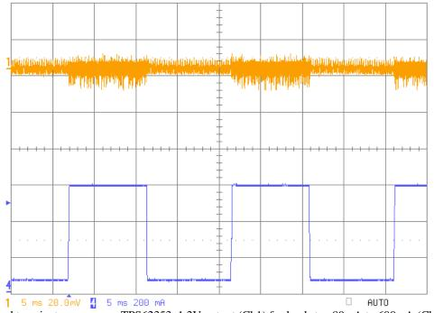
Fig 14: Load transient response on TPS62353, 1.2V output (Ch1) for load step 80mA to 600mA (Ch4 - 15% to 100%), at low line 3.6Vin
