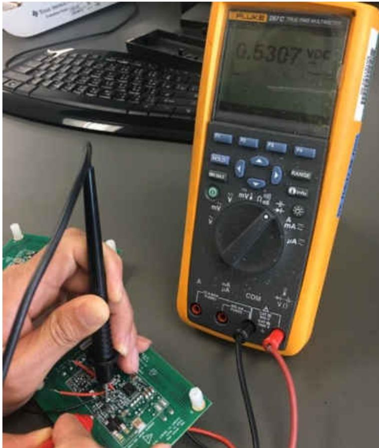
**Figure 1-1. Probing UCC28782 Pins with a Digital Multimeter**
