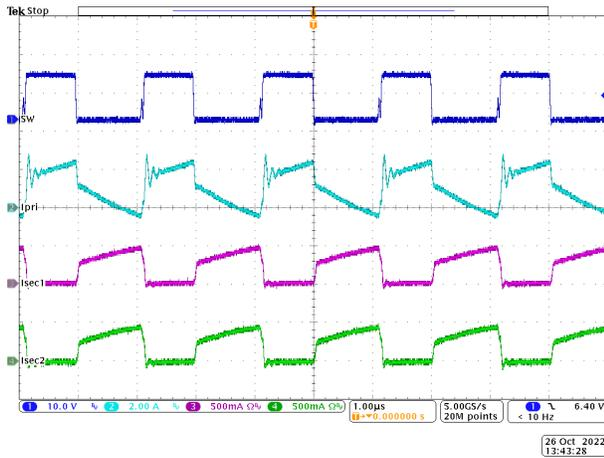
**Figure 4-1. Steady State Waveforms ( $V_{IN} = 10\text{ V}$ ,  $I_{OUT1} = 1\text{ A}$ ,  $I_{OUT2} = 0.2\text{ A}$ , and  $I_{OUT3} = 0.2\text{ A}$ )**
