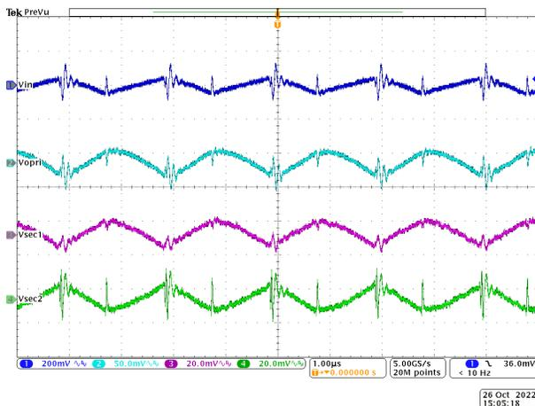
**Figure 4-3. Ripple Voltage Waveforms ( $V_{IN} = 10\text{ V}$ ,  $I_{OUT1} = 1\text{ A}$ ,  $I_{OUT2} = 0.2\text{ A}$ , and  $I_{OUT3} = 0.2\text{ A}$ )**
