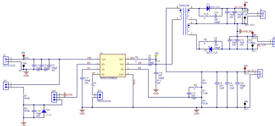
Figure 3-1. TPS62933F Two Output Isolated Buck Solution
