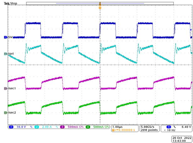
**Figure 4-2. Steady State Waveforms ( $V_{IN} = 10\text{ V}$ ,  $I_{OUT1} = 0\text{ A}$ ,  $I_{OUT2} = 0.2\text{ A}$ , and  $I_{OUT3} = 0.2\text{ A}$ )**
