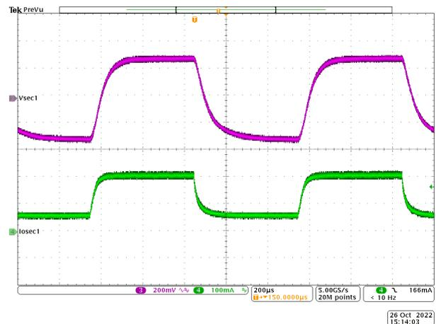
**Figure 4-4. Load Step Response 50 mA to 200 mA ( $V_{IN} = 10\text{ V}$ ,  $I_{OUT1} = 0\text{ A}$ , and  $I_{OUT3} = 0\text{ A}$ )**
