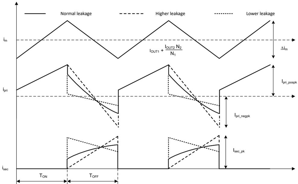
**Figure 2-3. Current Waveforms Affected by Leakage Inductance**
