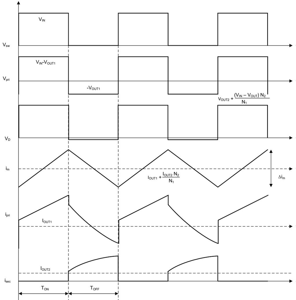
**Figure 2-2. Simplified Isolated Buck Operating Waveforms**
