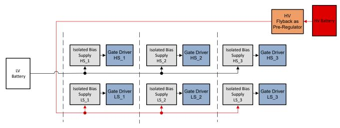
Figure 2-3. Pre-Regulator at High-Voltage Battery
