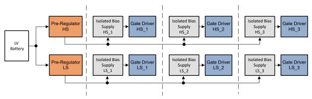
Figure 2-2. Two Pre-Regulators in a Fully-Distributed Architecture
