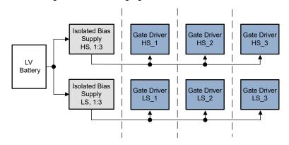
Figure 4-2. Semi-Distributed Architecture at High Side and Low Side
