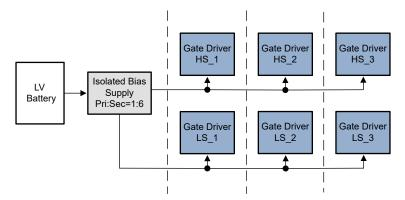
Figure 5-1. Centralized Architecture
