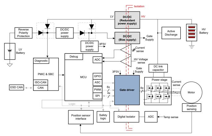
Figure 1-1. Traction Inverter Block Diagram
