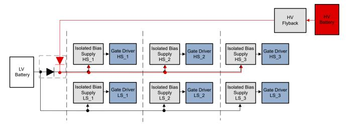
Figure 6-4. Redundancy Only at the High Side in Fully-Distributed Architecture
