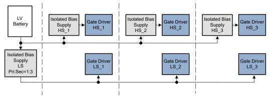
Figure 4-1. Semi-Distributed Architecture at Low Side Only
