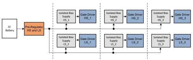
Figure 2-1. Single Pre-Regulator in a Fully-Distributed Architecture
