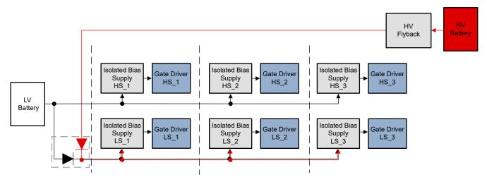
Figure 6-3. Redundancy Only at the Low Side in Fully-Distributed Architecture
