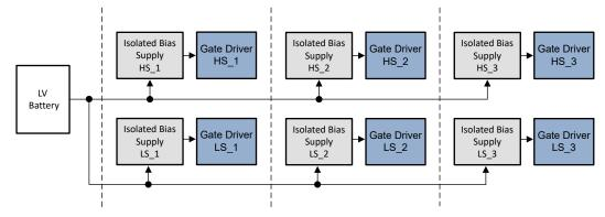
Figure 3-1. Fully-Distributed Architecture
