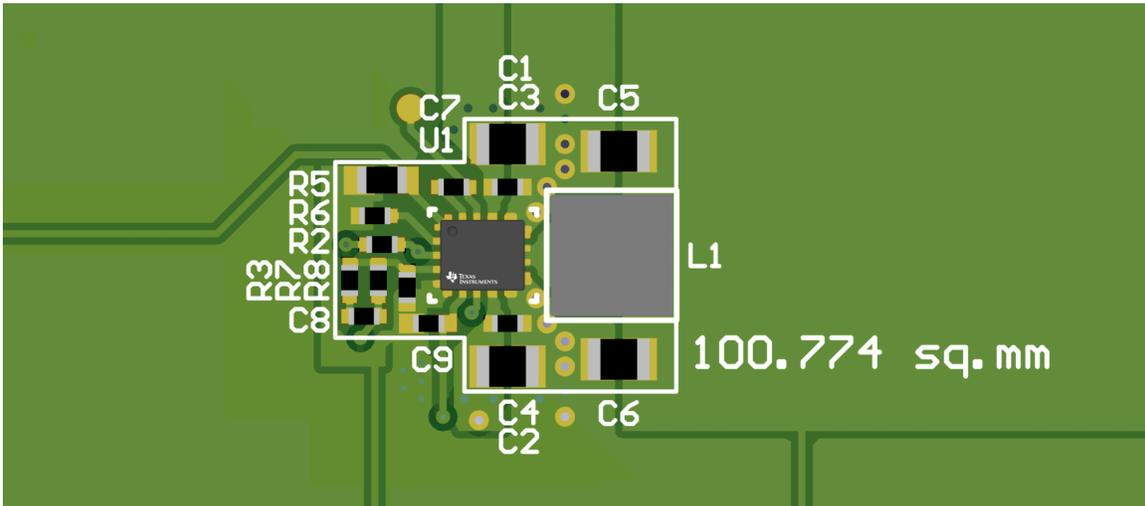
Figure 2-2. TPS543620 PCB Design Size
