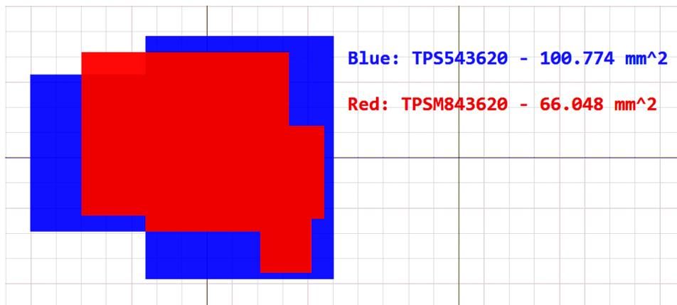
Figure 2-4. PCB Design Size Overlay Comparison
