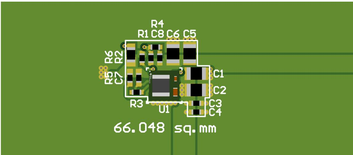
Figure 2-3. TPSM843620 PCB Design Size
