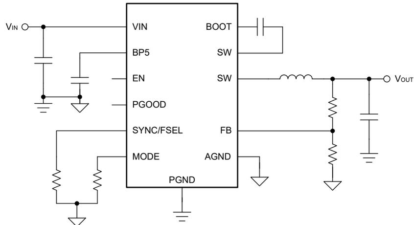
**Figure 2-5. TPS543620 Simplified Schematic**
