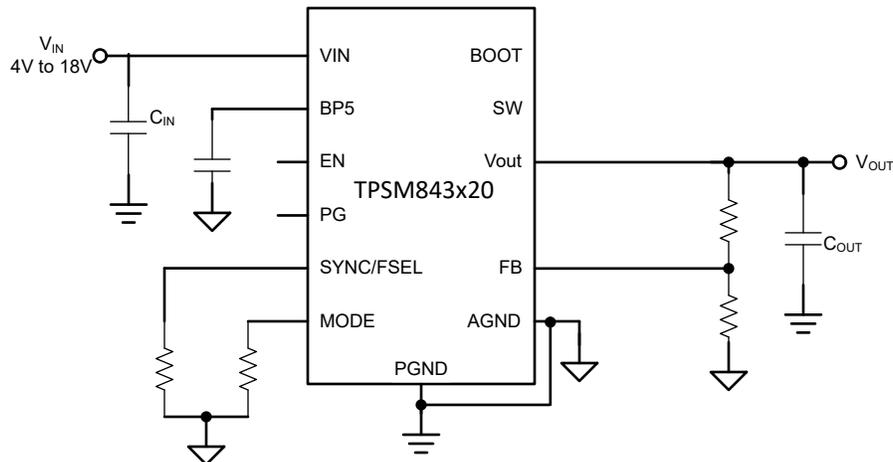
**Figure 2-6. TPSM843620 Simplified Schematic**
