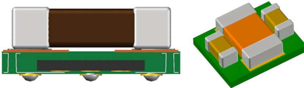
**Figure 2-1. MicroSiP Package Example**
