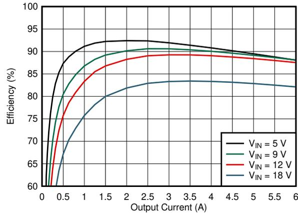
Figure 3-1. TPSM843620 Efficiency Graph
