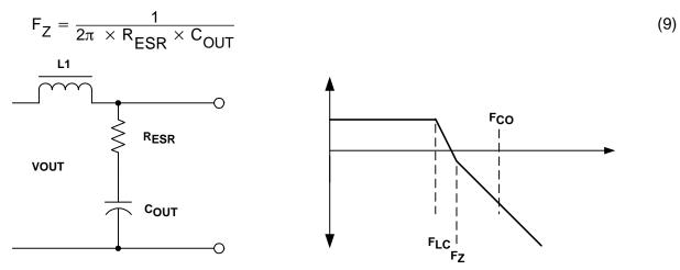
Figure 5. Output Filter with R<sub>ESR</sub> and Bode Plot.
