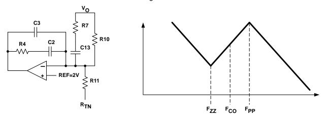
Figure 8. Error Amplifier with Two Pole-Zero Pairs
