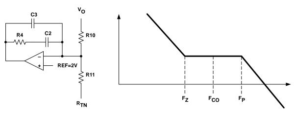
Figure 6. Error Amplifier with Zero-Pole Pair
