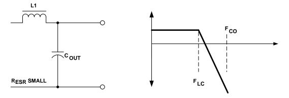
Figure 7. Output Filter with Negligible R<sub>ESR</sub>
