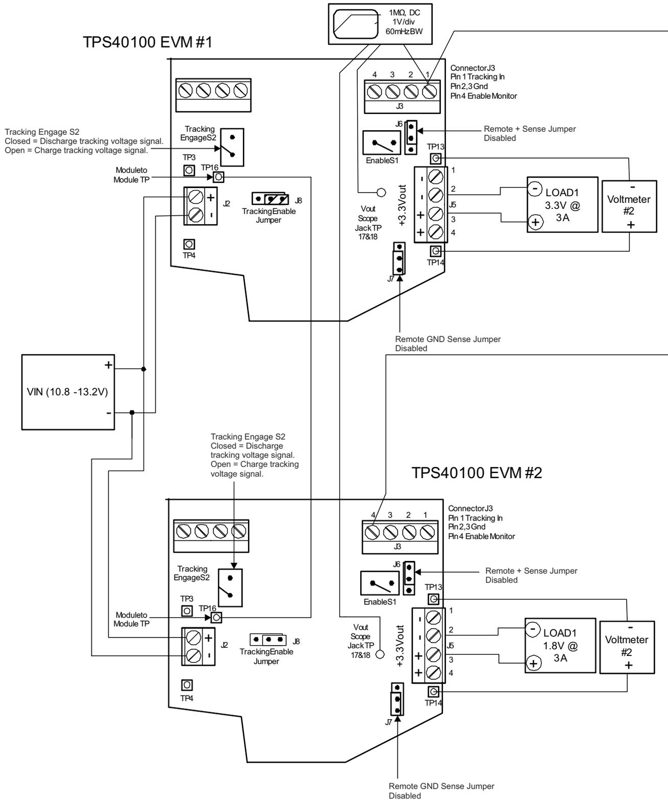
Figure 5-7. TPS40100EVM-001 Dual EVM Tracking Test Setup
