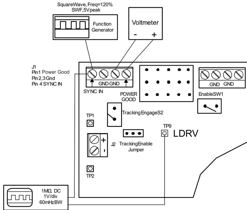
Figure 5-12. TPS40100EVM-001 Power Good and Synchronization Test Setup
