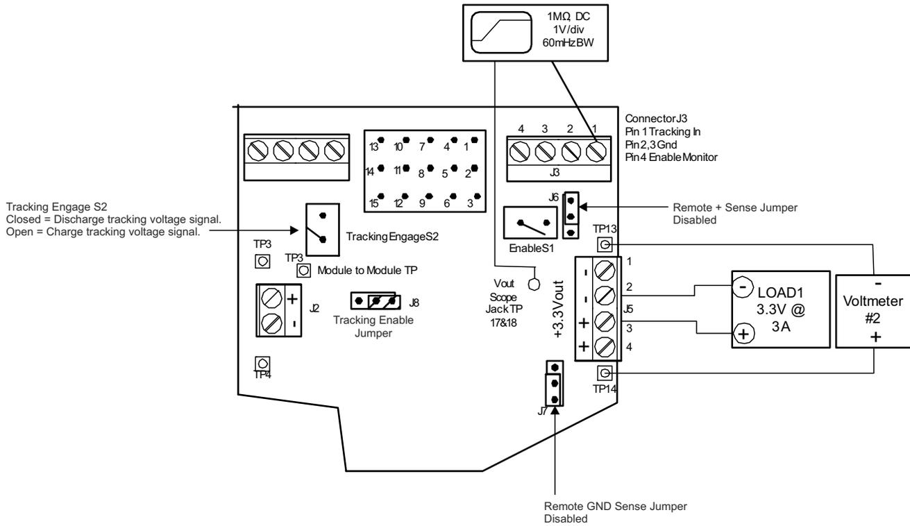
Figure 5-4. TPS40100EVM-001 Single EVM Tracking Test Setup
