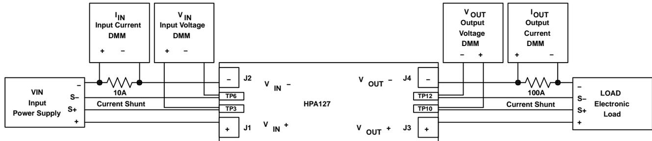
Figure 2. Recommended EVM test configuration.
