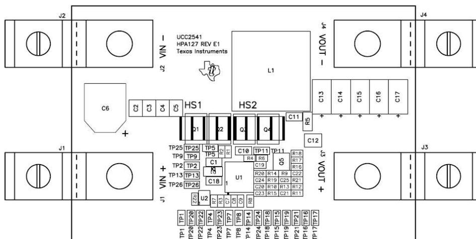
**Figure 3. Test Points for HPA127 Evaluation (TOP)**
