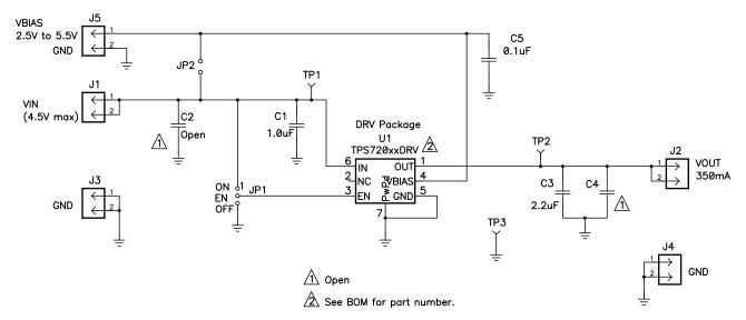
Figure 4. TPS720xxDRVEVM Schematic
