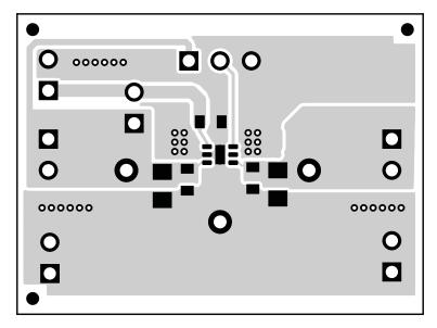
Figure 2. Top Layer Routing
