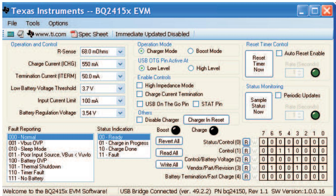
**Figure 3. Main Window of the bq2415x Evaluation Software**
