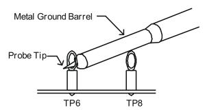
Figure 7-1. Tip and Barrel Measurement for V<sub>OUT</sub> Ripple
