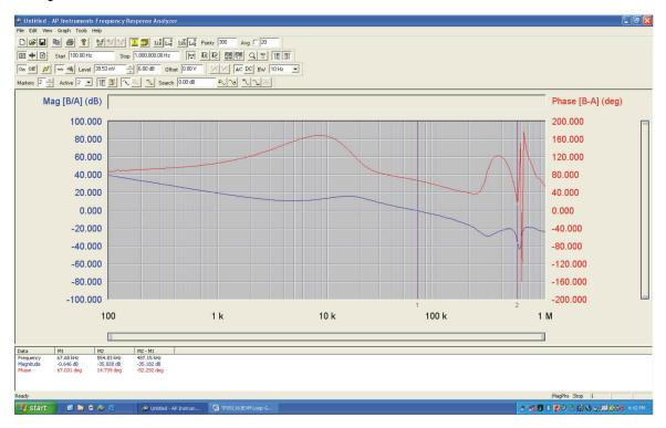
Figure 9-4. Loop Response Gain and Phase
