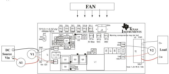
Figure 7-2. TPS51163EVM Recommended Test Setup
