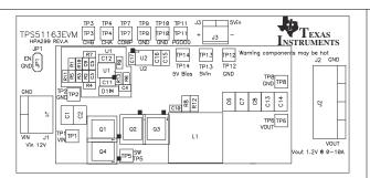
Figure 10-1. Top Layer Assembly Drawing (Top View)
