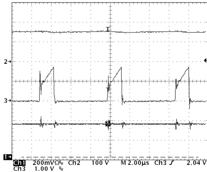
Figure 10. Line Voltage and Current Sense Waveform (peak line)
