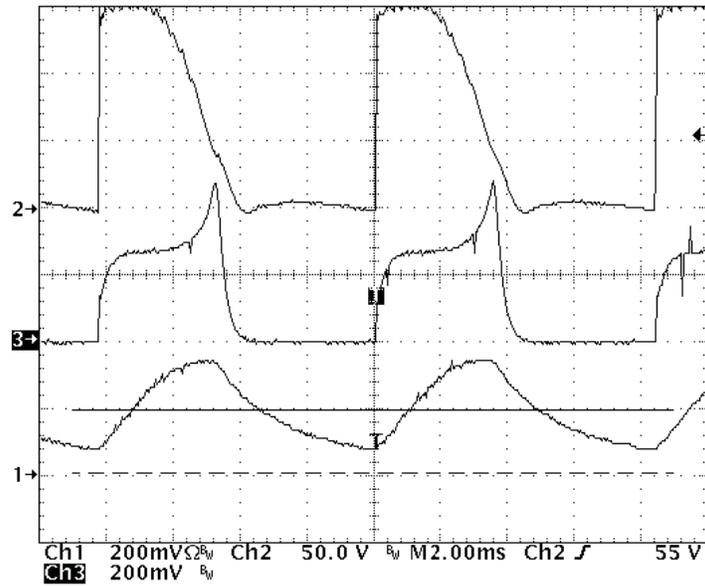
**Figure 25. LED Current vs. Triac Conduction Time**
