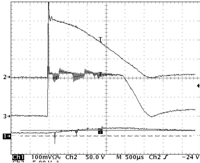
Figure 13. Triac Holding Current (2.5-ms Triac on time)
