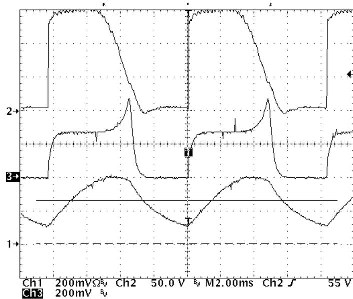
**Figure 26. LED Current vs. Triac Conduction Time**
