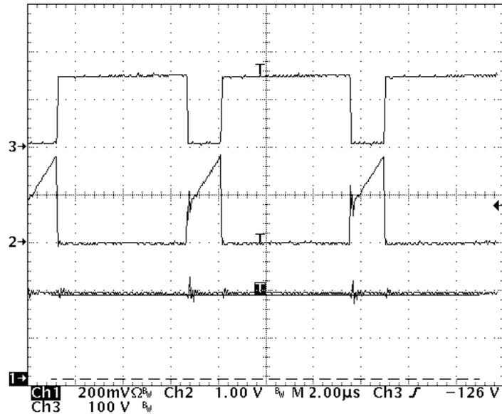
Figure 9. Current Sense and Switching Node Waveform (peak line)
