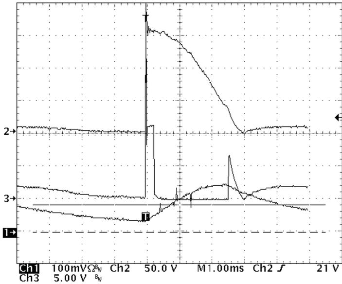
Figure 14. Triac Holding Current(3-ms Triac on time)
