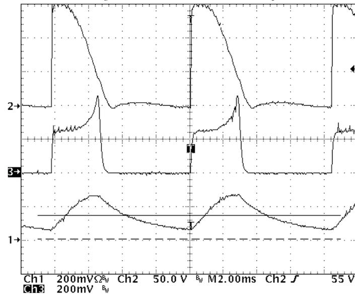
**Figure 24. LED Current vs. Triac Conduction Time**
