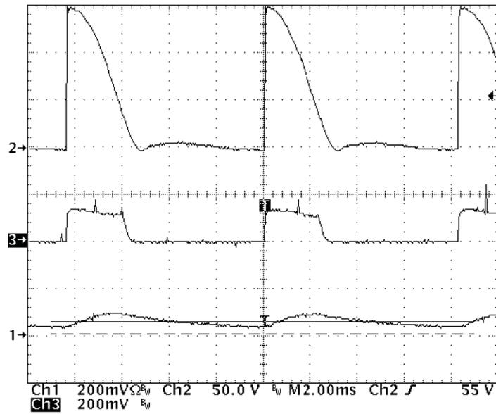
**Figure 23. LED Current vs. Triac Conduction Time**
