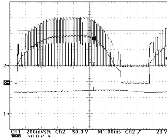
**Figure 11. LED Current vs. Q2 Switch Node**
