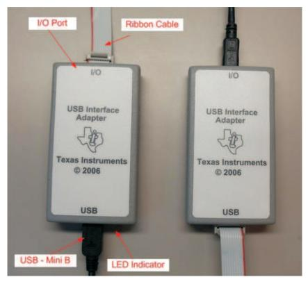
Figure 10. USB-to-GPIO Interface Adapter (HPA172)
