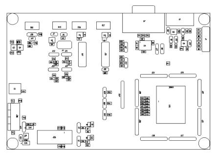
Figure 18. UCD3138OL64EVM-031 Top Layer Assembly Drawing (top view)
