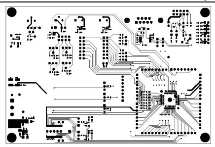
Figure 20. UCD3138OL64EVM-031Top Copper (top view)
