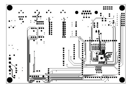
Figure 23. UCD3138OL64EVM-031 Bottom Copper (top view)
