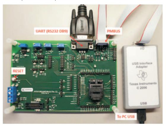
Figure 12. UCD3138OL64EVM-031 Test Connections
