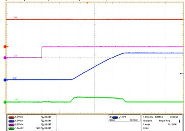
Figure 5-2. LM74900-Q1 Start-Up With EN - Output Voltage and Input Current Profile
