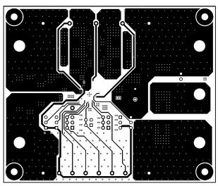
Figure 6-6. LM74900Q1EVM Board Inner Layer 2
