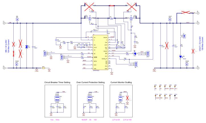
Figure 3-1. LM74900Q1EVM: Evaluation Module Schematic
