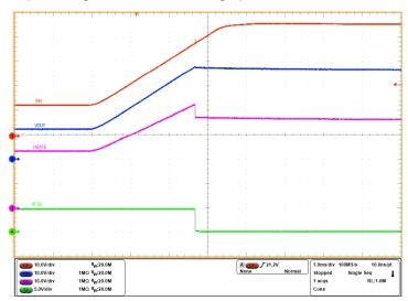
Figure 5-6. Overvoltage Protection
