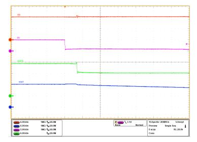
Figure 5-5. LM74900-Q1 Shutdown With EN - DGATE and Output Voltage Profile
