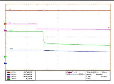
Figure 5-4. LM74900-Q1 Shutdown With EN - HGATE and Output Voltage Profile
