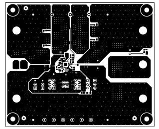
Figure 6-3. LM74900Q1EVM Board Top Layer
