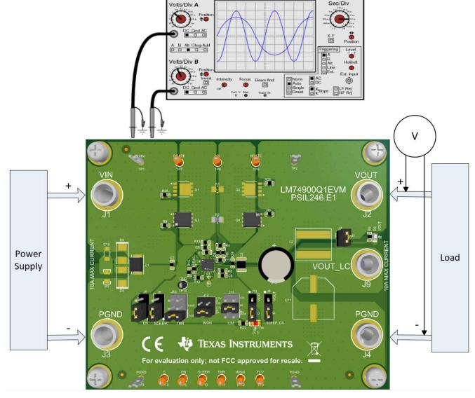
Figure 5-1. LM74900Q1EVM Setup With Test Equipment
