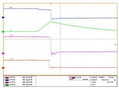
Figure 5-9. Output Hot-Short Response of LM74900-Q1 Device
