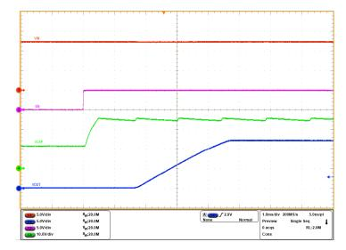
Figure 5-3. LM74900-Q1 Start-Up With EN - Charge Pump and Output Voltage Profile
