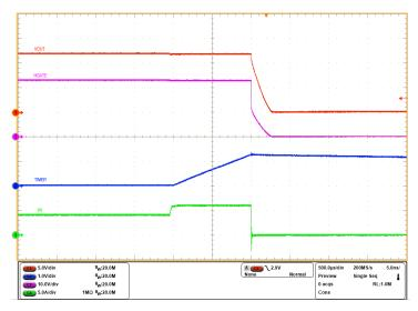
Figure 5-7. Overcurrent Response of LM74900-Q1 for a Load Step From 4 A to 6 A With 5-A Overcurrent Protection Setting
