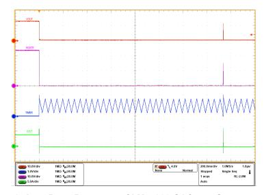
Figure 5-8. Auto-Retry Response of LM74900-Q1 for an Overcurrent Fault
