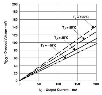
Figure 2. TPS799285 Dropout Voltage vs Output Current
