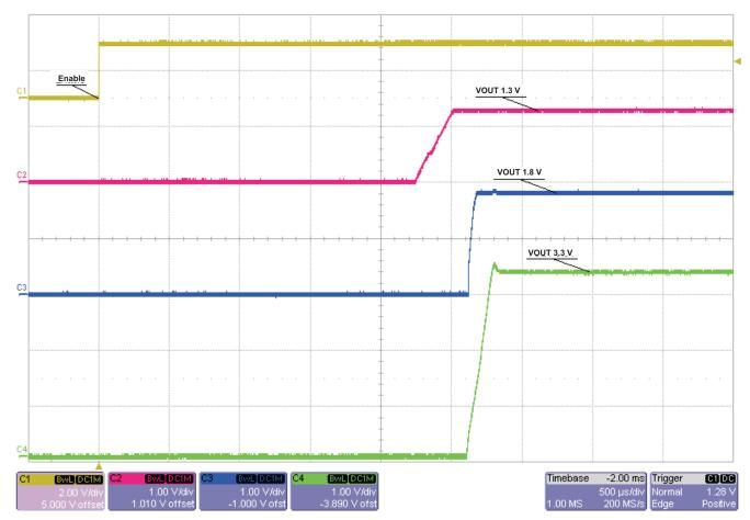
Figure 2. Power Up With 2-V Input and ENABLE Voltage
