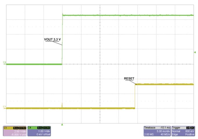
Figure 3. RESET Pin of TPS3808G33 Pulled High
