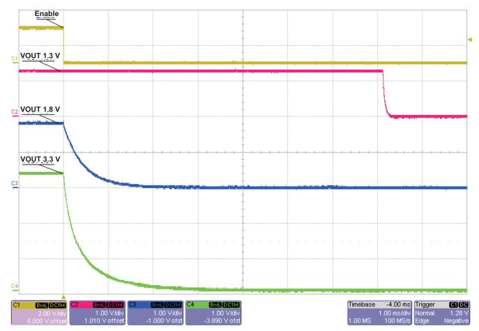
Figure 4. Power Down With 2-V Input and ENABLE Voltage
