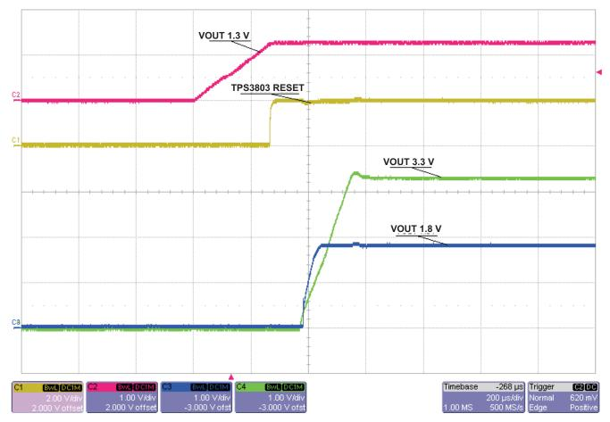
Figure 5. Power-Up Sequence Showing TPS3803-01 RESET Signal
