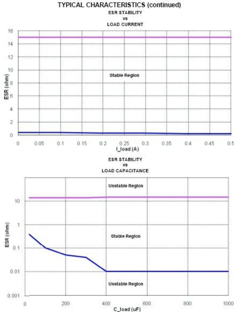
System designs must ensure their capacitor choice meets the published ESR limits for TLE4275 stability. When ceramic capacitors are used, a series resistor may be required to meet resistance minimum value. As an example, a 22  $\mu\text{F}$  ceramic capacitor with a .33- $\Omega$  series resistor will meet stability requirements over full temperature range.
