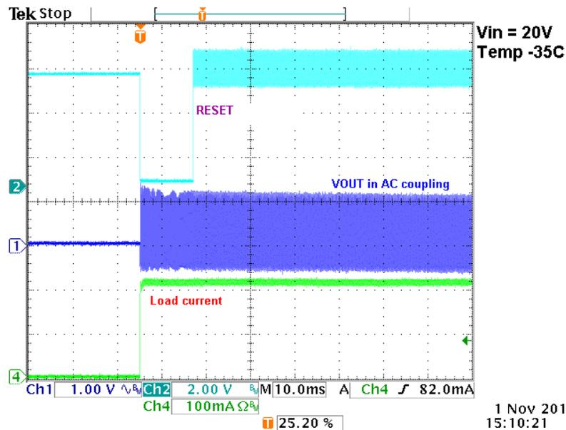
Oscilloscope trace 1 (blue) shows AC coupled output voltage  $V_{OUT}$ , trace 2 (aqua) reset pin voltage, trace 4 (green) load current. Note that voltage is not stable as device is enabled; there are large-amplitude, high-frequency oscillations.
