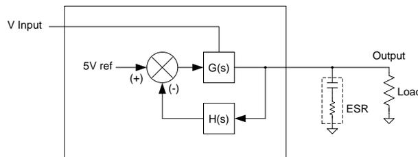
For the most common applications, an electrolytic output capacitor is used, and the low temperature stability issue can be traced to an increase in its equivalent series resistance (ESR) at low temperature. The additional resistance introduces changes in the system transfer function which are beyond the limits of stability.
