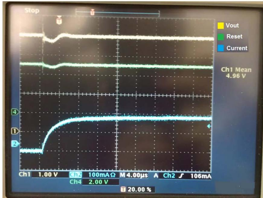
Figure 2. 68µF/16V Panasonic EEE-FT Series Cap at  $V_{IN} = 20V$
