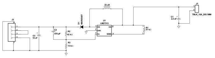
$V_{\text{IN}}$  = 3 V to 5 V,  $V_{\text{OUT}}$  = 5V,  $I_{\text{OUT}}$  = 500 mA
