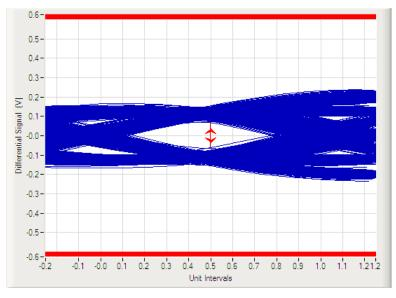
Figure 4. USB 3.1 Gen 2 10-Gbps Eye Diagram (Bare Board)
