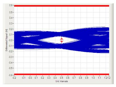
Figure 5. USB 3.1 Gen 2 10-Gbps Eye Diagram (with TPD1E01B04)
