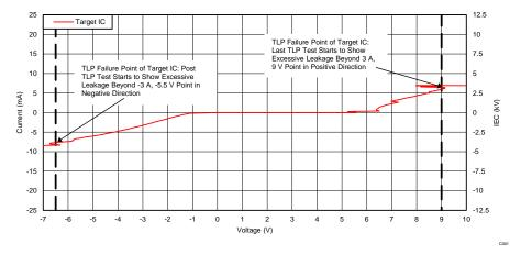
Figure 1. TLP Measurement Example
