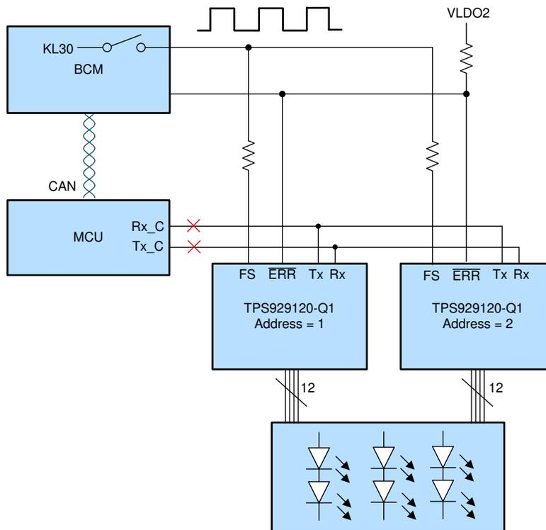
Figure 10. Turn Indicator System Block Diagram in Fail-Safe State
