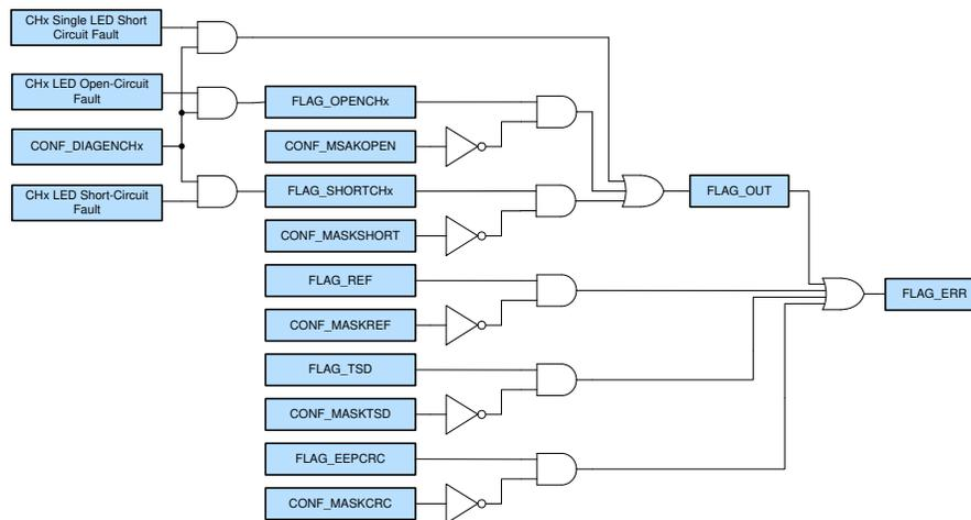
Figure 5. Diagnostic Enable and Fault Mask
