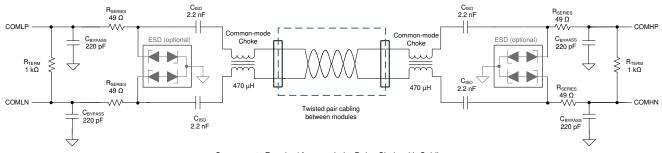
Components Required for cap-choke Daisy Chain with Cabling
