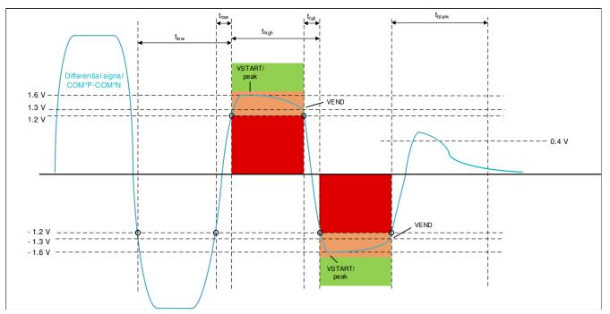
Figure 3-2. Differential Signal Eye Diagram - 1.6 V VSTART
