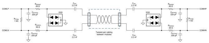
Components Required for Cap Coupled Daisy Chain on different pcb
