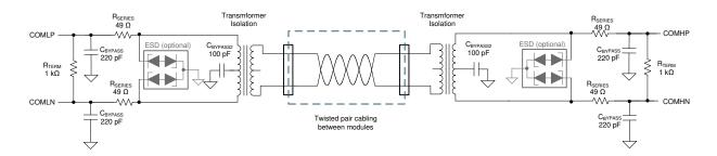
Figure 5-1. Transformer Isolation Across PCBs
