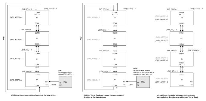
Figure 7-1. Example to Change Communication Direction in Daisy Chain
