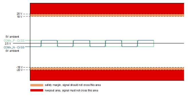
Figure 2-1. Common Mode Voltage Diagram
