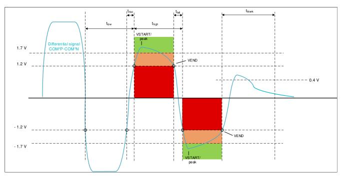
Figure 3-1. Differential Signal Eye Diagram - 1.7 V VSTART
