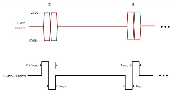
Figure 1-3. Daisy Chain Bit Level Definition
