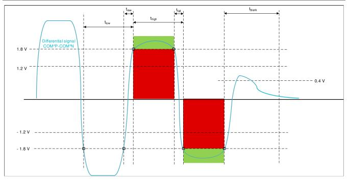
Figure 3-3. Differential Signal Eye Diagram - BQ79600
