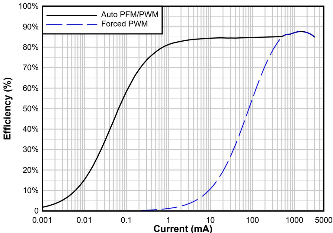
**Figure 2-1. Efficiency Comparison at Auto PFM/PWM vs FPWM**
