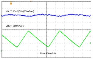
Figure 4-7. TPS61099 Vin 3.6 V ,Vout 5 V, lout 300 mA
