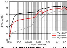
Figure 4-3. TPS61299 Efficiency ,Vout=5 V
