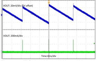
Figure 4-5. TPS61099 Vin 3.6 V, Vout 5 V, Iout 0A
