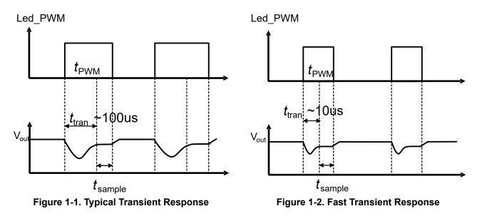
Assuming the sample times being equal, with fast transient performance shown in Figure Figure 1-2, the  $t_{tran}$  can be reduced from 100 us to 10 us, thus the period of Led\_PWM can be reduced as well, denoted as  $t_{PWM}$ . With reducing LED light time, the system reduces energy consumption and improves its efficiency.
