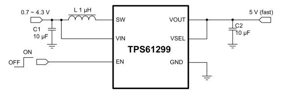
Figure 2-1. Schematic of TPS61299 Power Supply Under 5 V Vout Fast Transient Mode
