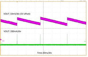
Figure 4-8. TPS61299 Vin 3.6 V ,Vout 5 V, lout 0 A
