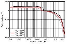
Figure 4-4. TPS61299 Load Regulation ,Vout=5V
