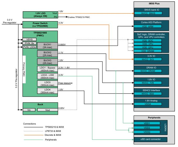
Figure 3-2. Powering i.MX 8M Plus and LDDR4 - Supports SNVS Low Power Mode
