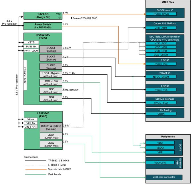
Figure 3-1. Powering i.MX 8M Plus and DDR4 - Supports SNVS Low Power Mode
