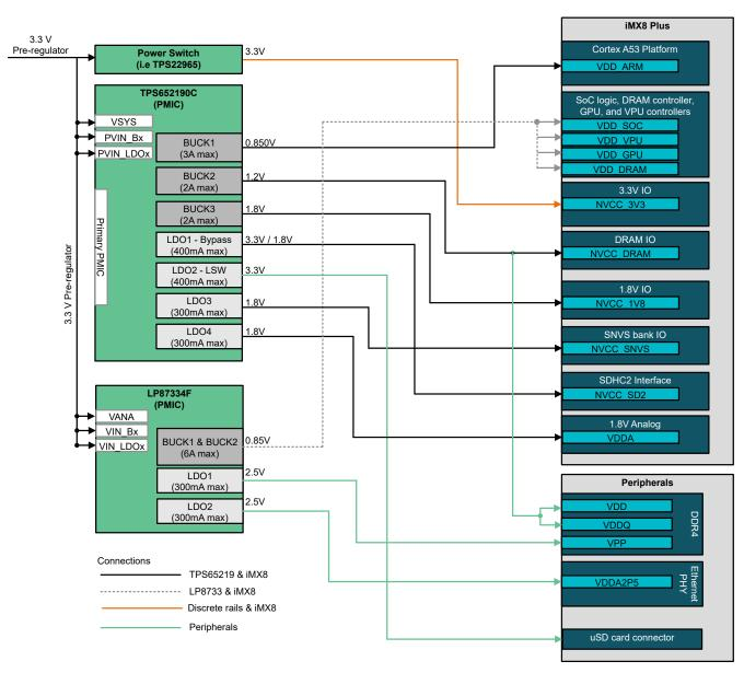
Figure 2-1. TPS652190C Powering i.MX 8M Plus and DDR4
