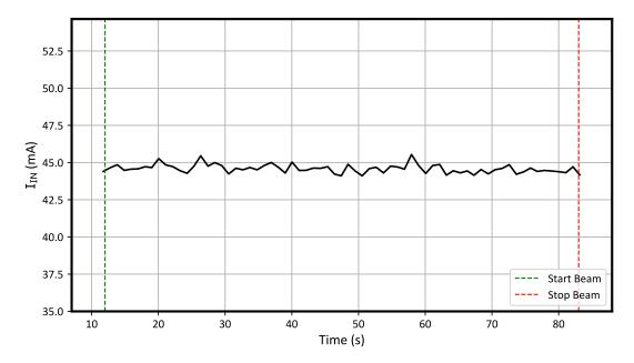
Figure 7-4. Current vs Time for Run #6 (Enabled) for the TPS7H1111-SEP at T = 25°C (0.4-V)
