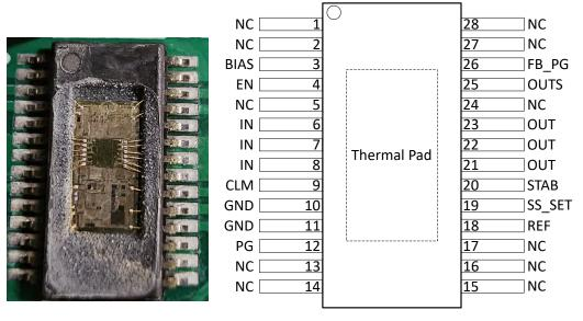
Figure 3-1. Photograph of Exposed TPS7H1111-SEP [Left] and Pinout Diagram [Right]
