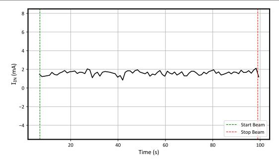
Figure 7-3. Current vs Time for Run #5 (Disabled) for the TPS7H1111-SEP at T = 25°C (0.4-V)
