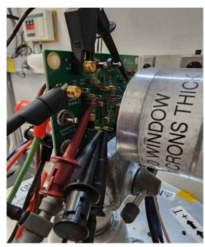
Figure 4-1. Photograph of the TPS7H1111-SEP EVM in Front of the Heavy-Ion Beam Exit Port at the Texas A&M Cyclotron
