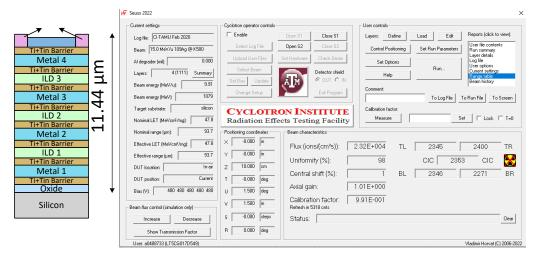
Figure 5-1. Generalized Cross-Section of the LBC7 Technology BEOL Stack on the TPS7H1111-SEP [Left] and SEUSS 2022 Application Used to Determine Key Ion Parameters [Right]
