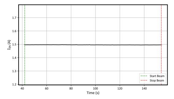
Figure 7-6. Current vs Time for Run #10 (Enabled) for the TPS7H1111-SEP at T = 25°C (5.5-V)
