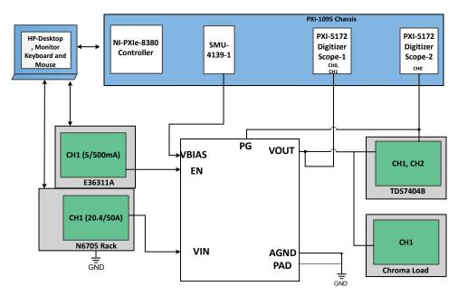
Figure 6-1. Block Diagram of the SEE Test Setup for the TPS7H1111-SEP
