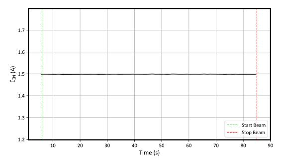
Figure 7-2. Current vs Time for Run #3 of the TPS7H1111-SEP at T = 125°C (5.5-V)
