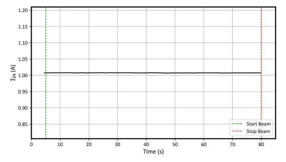
Figure 7-1. Current vs Time for Run #1 of the TPS7H1111-SEP at T = 125°C (0.4-V)
