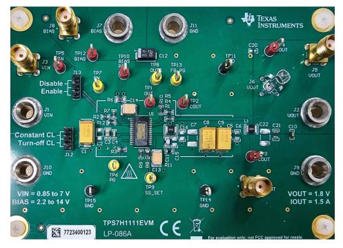
Figure 3-2. TPS7H1111-SEP SEE Test Board Top View
