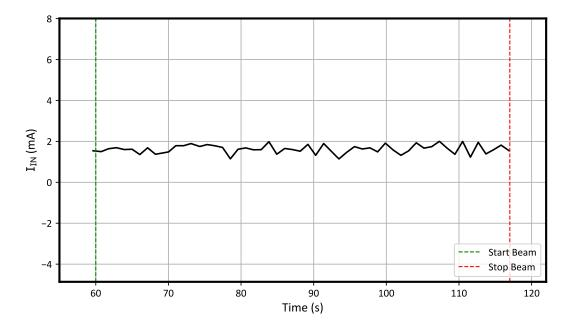
Figure 7-5. Current vs Time for Run #9 (Disabled) for the TPS7H1111-SEP at T = 25°C (5.5-V)
