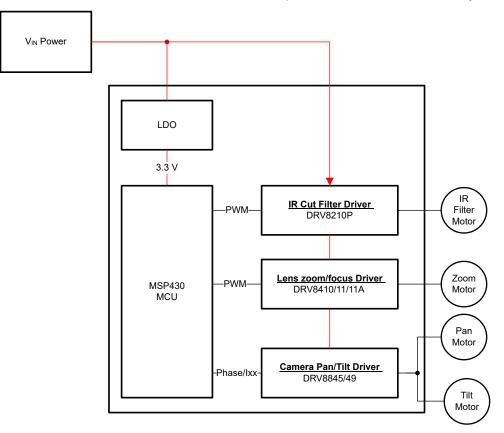
Figure 1. Video Surveillance Motor Drive Applications
