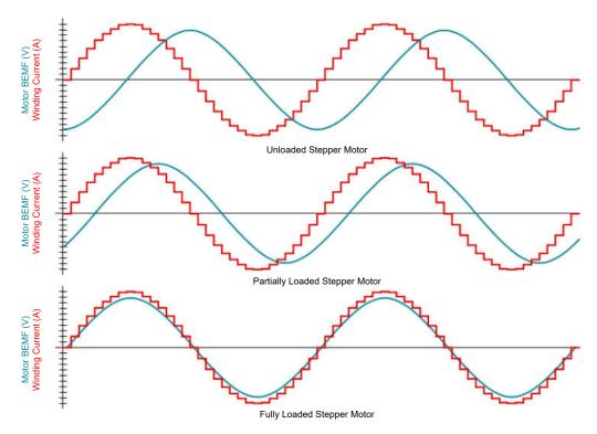
Figure 4. Stall Detection by Monitoring Motor Back-EMF
