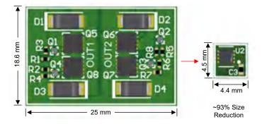
Figure 2. Discrete vs DRV8210 and DRV8220 Layout Size
