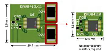
Figure 3. Integrated Current-Sensing Size Comparison on DRV8411A
