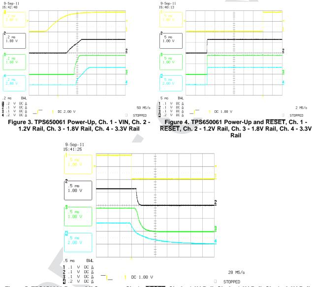
Figure 5. TPS650061 Power-Off Sequence, Ch. 1 - RESET, Ch. 2 - 1.2V Rail, Ch. 3 - 1.8V Rail, Ch. 4 - 3.3V Rail
