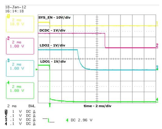
Figure 5. Power-Down Sequence With System Enable LOW
