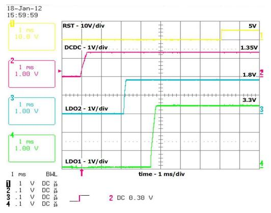
Figure 4. Power-Up Sequence and Reset Release
