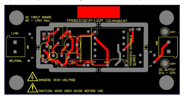
Figure 11. Top Layer and Top Overlay (Top view)
