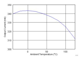
Figure 5. Output Current versus Temperature
