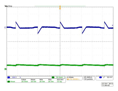
Figure 8. Triac Minimum Level Waveform
