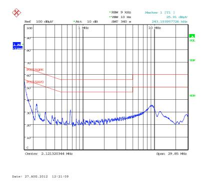
Figure 9. 120VAC Line-Conducted Average EMI Scan
