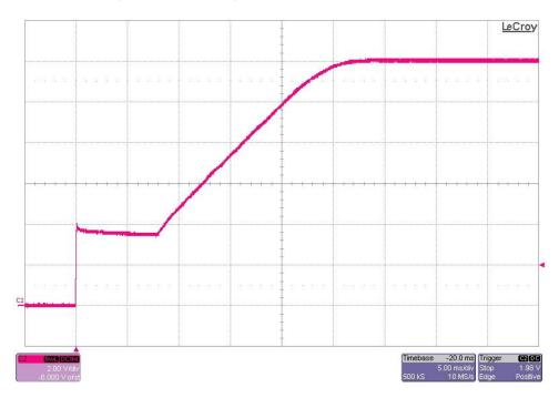
The photo below shows the output voltage startup waveform after the application of 3.8V in. The 12V output was loaded to 4A. (2V/DIV, 5mS/DIV)
