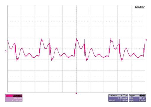
The 12V output ripple voltage is shown in the figure below. The image was taken with the output loaded to 4A. The input voltage is set to 7.6V. (100mV/DIV, 2uS/DIV)
