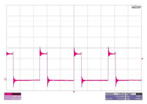
The photo below shows the FET switching voltage. The input voltage is 3.8V and the output is loaded to 4A. (5V/DIV, 2uS/DIV)
