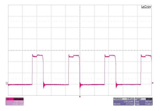
The photo below shows the FET switching voltage. The input voltage is 7.6V and the output is loaded to 1A. The boost converter is starting discontinuous mode operation. (5V/DIV, 2uS/DIV)
