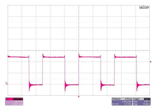
The photo below shows the FET switching voltage. The input voltage is 8.6V and the output is loaded to 4A. (5V/DIV, 2uS/DIV)
