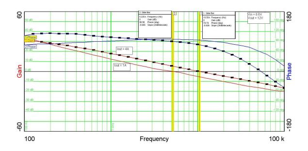
The plot below shows the loop gain and phase margin with the output loaded to 1A and 4A. The input voltage was set to 7.6V.
