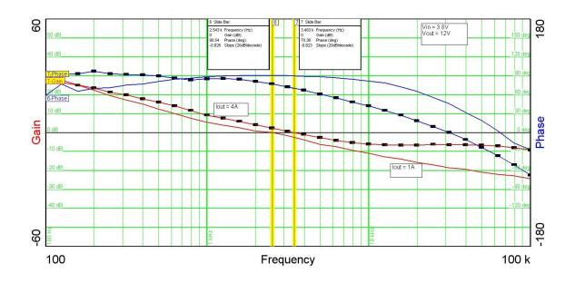
The plot below shows the loop gain and phase margin with the output loaded to 1A and 4A. The input voltage was set to 3.0V.
