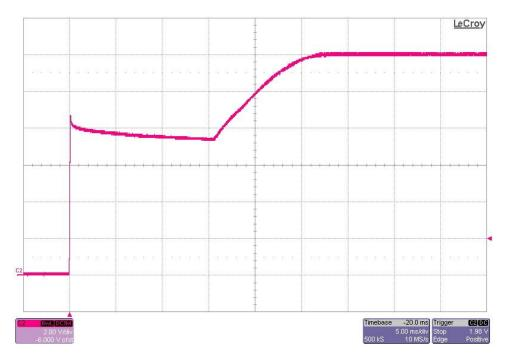
The photo below shows the output voltage startup waveform after the application of 7.6V in. The 12V output was loaded to 4A. (2V/DIV, 5mS/DIV)
