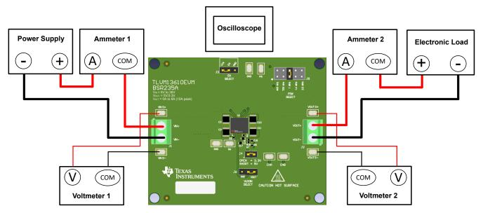
Figure 2-1. EVM Test Setup
