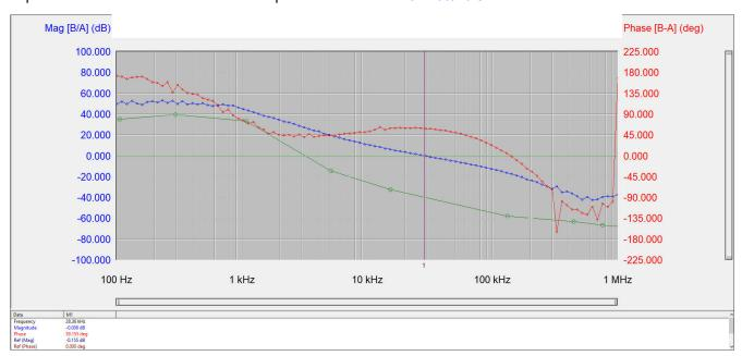
Figure 3-13. Bode Plot With Four 47-μF, 16-V Output Capacitors (110 μF Effective at 5 VDC, 25°C)
