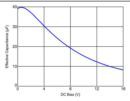
Figure 3-14. Output Capacitor Voltage Derating Curve
