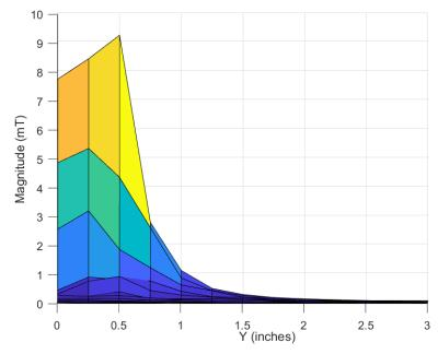
Figure 3-4. TMAG5273 Magnet 1 Detection Field (2D)
