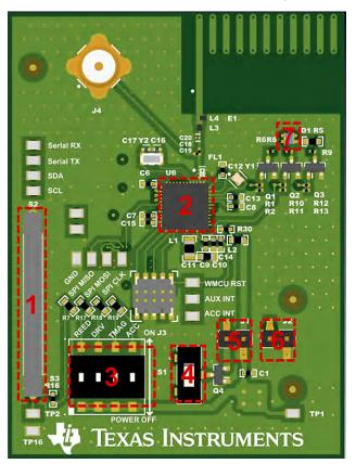
Figure 2-2. Door and Window Sensor Evaluation Platform Top View
