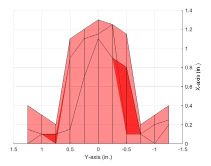
Figure 3-10. Reed Switch Magnet 2 Detection Field (2D Top Down)
