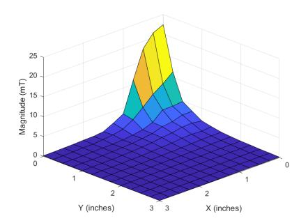
Figure 3-9. TMAG5273 Magnet 2 Detection Field (3D)
