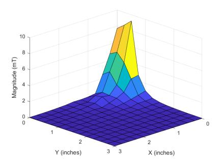
Figure 3-5. TMAG5273 Magnet 1 Detection Field (3D)
