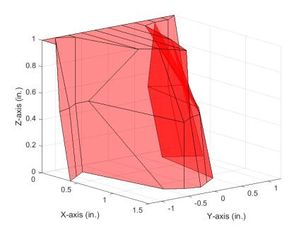
Figure 3-11. Reed Switch Magnet 2 Detection Field (3D)
