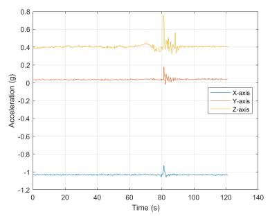
Figure 3-13. Accelerometer Door Close Event
