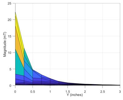
Figure 3-8. TMAG5273 Magnet 2 Detection Field (2D)
