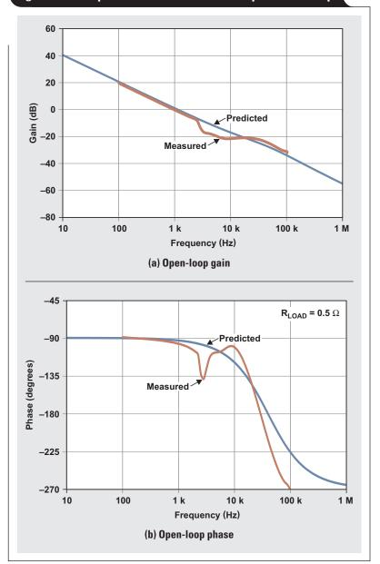
Figure 7. Bode plot of converter's final compensation loop
