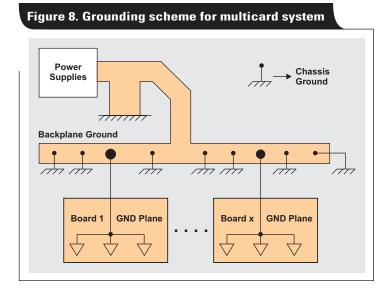
ground impedance is maintained all the way through the PCBs, the backplane, and ultimately the chassis. However, it is critical that good electrical contacts be made where the grounds are connected to the sheet-metal chassis. This requires self-tapping sheet-metal screws or biting washers. Special care must be taken where anodized aluminum is used for the chassis material, since its surface acts as an insulator.
