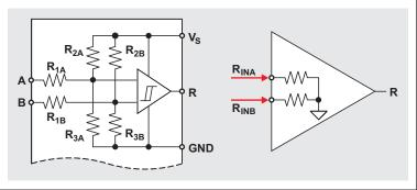
Because  $R_{FS}$  in combination with  $R_{INEQ}$  makes up the total common-mode load for a signal line, the parallel value of the two must not exceed the specified maximum of 375  $\Omega$ , which is expressed through
