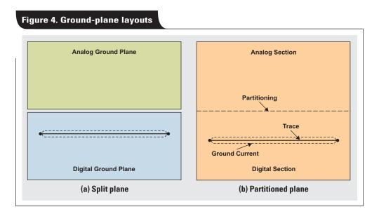
into analog and digital sections (see Figure 4b). Analog signals must be routed only in the board's analog section, and digital signals must be routed only in the board's digital section, with both on all layers. Under these conditions, the digital return currents do not flow in the analog section of the ground plane and remain under the digital signal trace. Figure 4 compares a split plane and a partitioned plane.
