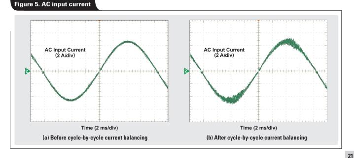
the same duty-ratio adjustment is applied to the next half AC cycle. This essentially solves the issue of high-frequency noise. Test results showed that the AC current's waveform was almost the same as before current balancing was enabled; the high-frequency noise went away.
