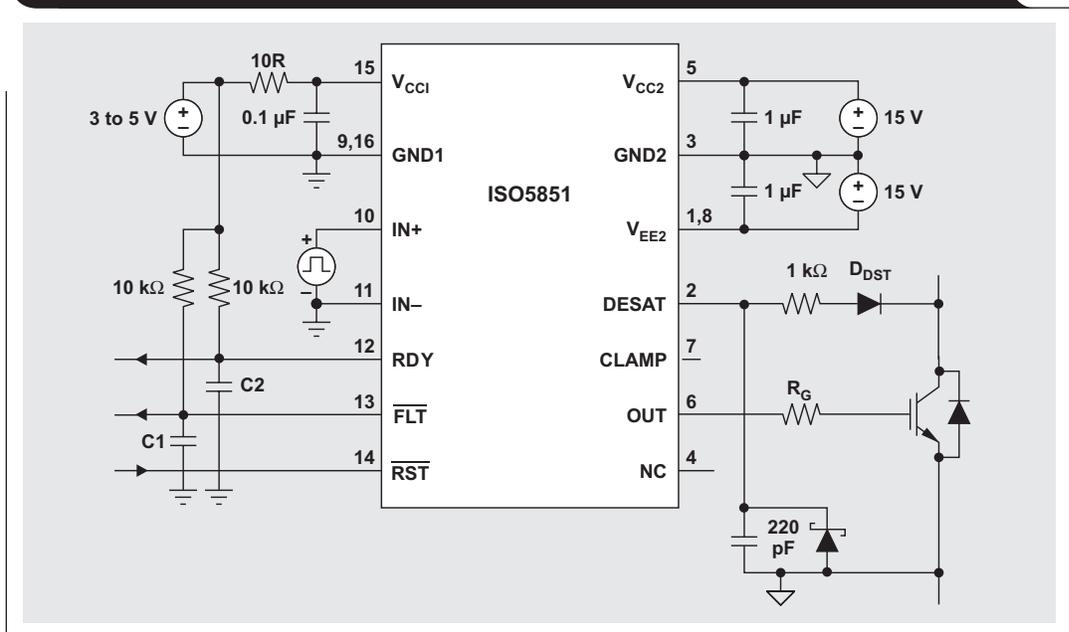
**Figure 8. Gate-driver solution using digital isolators**
