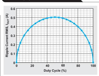
Figure 4. Input RMS/Load current ratio versus duty cycle
