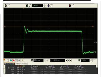
There could be two  $V_{IN}$  spikes during the transient: the first spike is related to the  $ESR_B$ ; and the second spike is caused by the difference between the buck-converter input current ( $\widetilde{i}_{IN\_D}$ ) and the bus-converter output current ( $i_{PS}$ ). Both spikes should be lower than the  $V_{IN}$  undershoot or overshoot requirement ( $V_{IN\_tran}$ ).
