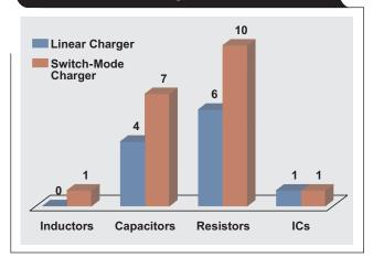
The lower BOM count in a linear charger can translate into application area savings. Any passive elements not used saves space needed for the charger. An inductor is not needed in a linear charger, which also saves space as shown in Figure 5. In low-power applications where space is critical, linear chargers can be a better fit.
