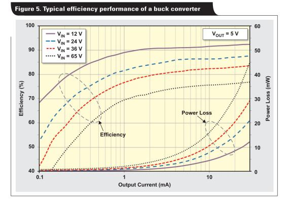
The total current budget must be sufficient to power all functional blocks of the transmitter: sensor interface and excitation, linearization method (MCU), galvanic barrier jump (if needed), 4–20-mA loop driver, and so forth. The solution presented was an integrated and robust DC/DC buck converter that has ultra-high efficiency across wide supply-voltage and load-current ranges. The resulting compact solution was achieved with minimal design effort.
