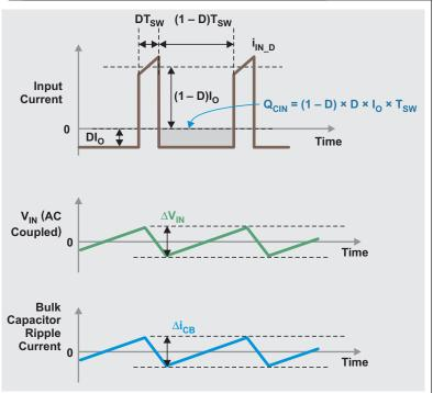
However, the criterion for the product of the allowable ripple current and the  $\mathrm{ESR}_{\mathrm{B}}$  remains the same. If no electrolytic capacitor meets the ripple-current requirement, extra ceramic capacitors are necessary. The extra ceramic capacitance can be estimated by solving Equations 8 and 9.
