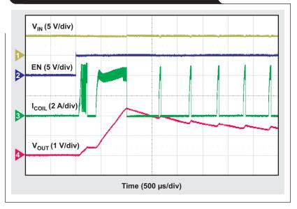
converge to create a system-startup issue. Figure 1 shows the startup of a power module with a 5-V input voltage, the output voltage set to 2.5 V, and two 470-µF capacitors added to the output.<sup>[1]</sup> With a 1-A resistive load added to the output, the output voltage never enters regulation because of current-limit and hiccup current-limit protection. Thus, the device remains in hiccup currentlimit operation.
