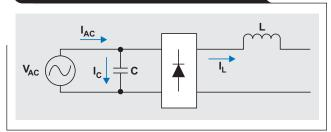
A power supply with PFC has two purposes. The first is to rectify the AC voltage ( $V_{AC}$ ) into a DC voltage ( $V_{OUT}$ ) and maintain  $V_{OUT}$  at a specific level. The second is to control the input current to follow the input voltage so that a good PF can be achieved. With the ever increasing PF requirements, especially in the server and telecommunications industries, it is a design challenge for a PFC to achieve an excellent PF with traditional control methods.
