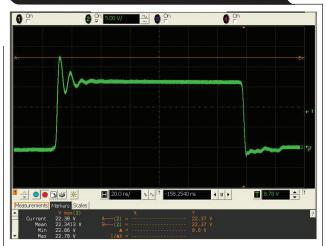
For phase-node ringing, it is common practice to use a boot resistor to slow down the gate speed and a snubber circuit for alleviation. However, both methods incur additional power loss and sacrifice efficiency. Phase-node ringing can be reduced without the penalty of lower efficiency.
