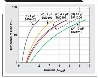
Since the board temperature is 75°C and the X5R MLCC is rated for 85°C, capacitor temperature rise should be lower than 10°C. Figure 5 shows the temperature rise characteristics of different ceramic capacitors.
