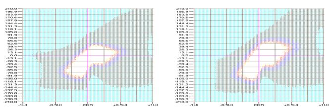
Figure 3. Receive Eye of 10.3125-Gbps Serialized Data with Oscillator (Left) and LMK03328 (Right)
