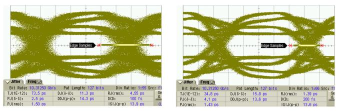
Figure 2. Transmit Eye of 10.3125-Gbps Serialized Data with Oscillator (Left) and LMK03328 (Right)
