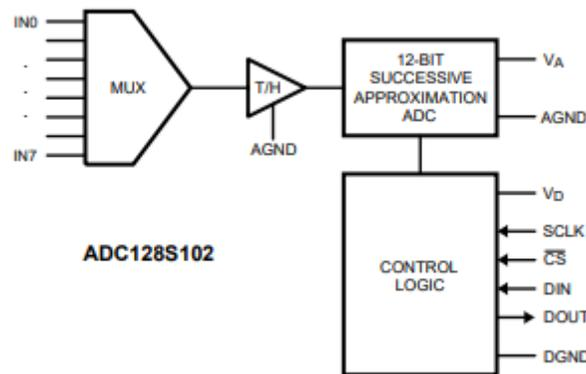
Figure 2-1. Functional Block Diagram of the ADC128S102-SEP
