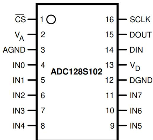
Figure 3-1. ADC128S102-SEP Pinout Diagram
