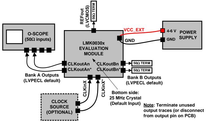
Figure 2: LMK00304 Evaluation Board Quick Start Setup
