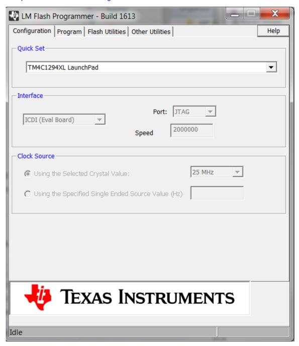
Figure 7. TM4C1294 LaunchPad™ selection in Configuration Tab
