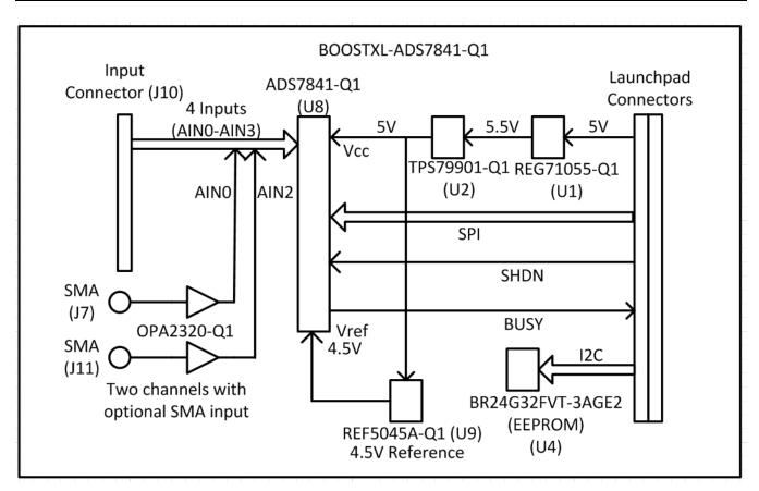
Figure 1. BOOSTXL-ADS7841-Q1 EVM Block Diagram
