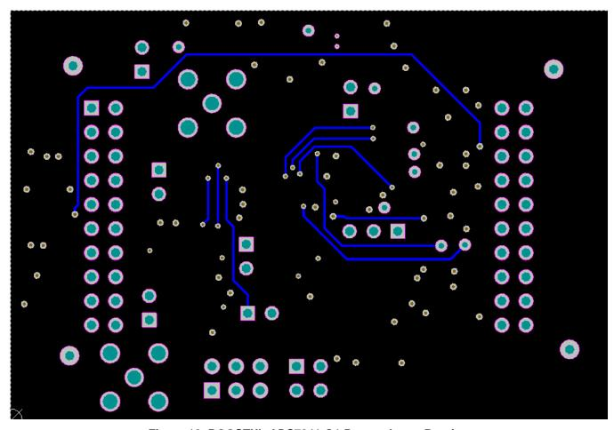
Figure 18. BOOSTXL-ADS7841-Q1 Bottom Layer Routing
