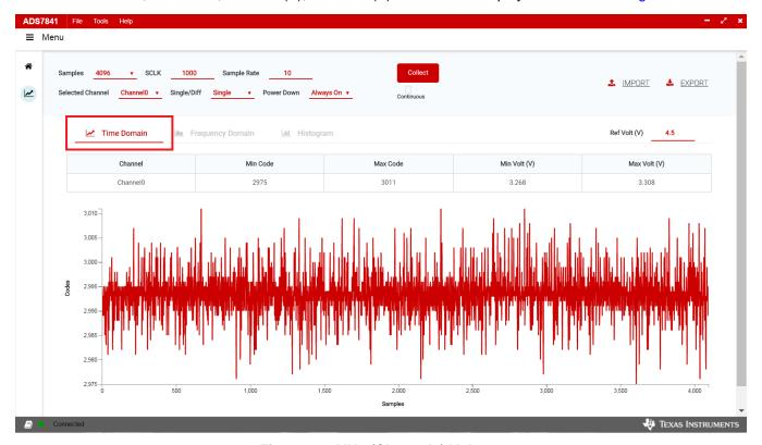
Figure 12. AIN0 (Channel0) Voltage
