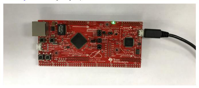
Figure 6. TM4C1294 LaunchPad™ Software Programming Setup
