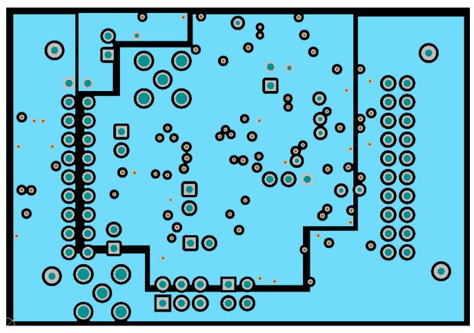
Figure 17. BOOSTXL-ADS7841-Q1 Power Layer
