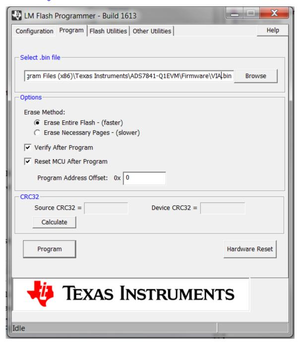
Figure 8. TM4C1294 LaunchPad™ Programming Using LM Flash Programmer
