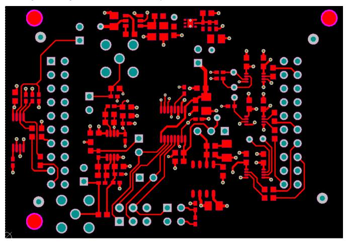
Figure 15. BOOSTXL-ADS7841-Q1 Top Layer Routing
