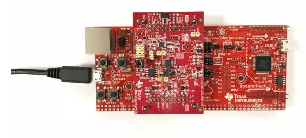
Figure 10. BOOSTXL-ADS7841-Q1EVM stacked on TM4C1294 LaunchPad™
