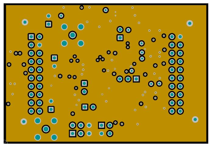
Figure 16. BOOSTXL-ADS7841-Q1 Ground Layer
