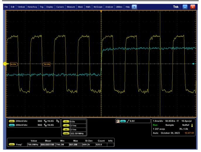
Figure 4-5. 800-MHz Buffer Mode With 10 MHz SYSREF
