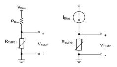
Figure 2. Thermistor Current and Voltage Biasing Circuits
