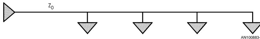
FIGURE 1. Daisy Chain Bus Configuration Supports Multi-drop Applications
