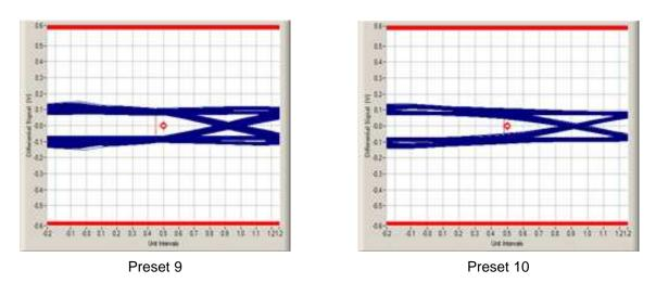
Figure 12. Non-Transition Eye Diagrams
