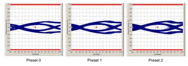
Figure 5. Transition Eye Diagrams
