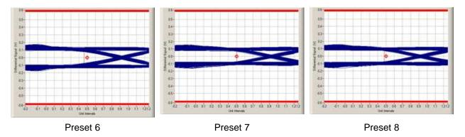
Figure 11. Non-Transition Eye Diagrams
