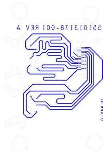
Figure 7. Passive Adapter Board Layout (Bottom View)
