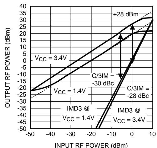
Figure 2. Linearity of CDMA RF Power Amplifier
