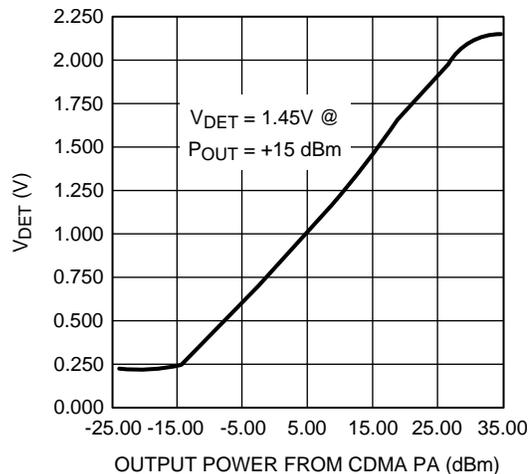
**Figure 4. LMV225 Detected Voltage vs.  $P_{OUT}$**
