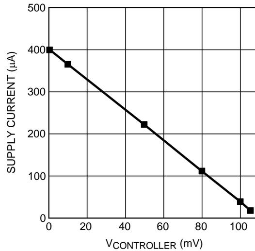
Figure 3. Power-Mode Control ( $R_{EXT} = 20\Omega$ ).
