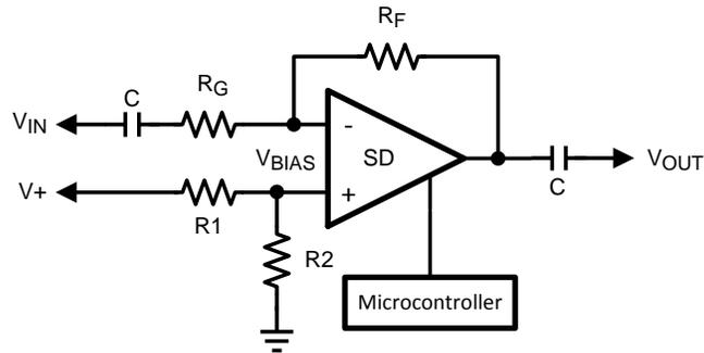
**Figure 1. AC-Coupled Inverting Amplifier With Shutdown Pin**
