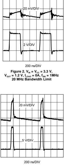
Figure 4.  $V_{IN}$  = 14 V,  $V_{cc}$  = 5 V,  $V_{OUT}$  = 1.2 V,  $I_{LOAD}$  = 0A,  $f_{SW}$  = 1MHz. 20 MHz Bandwidth Limit
