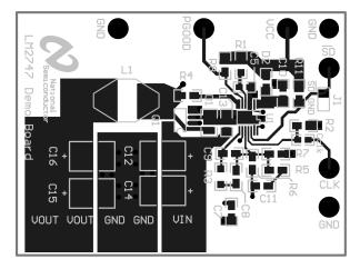
Figure 7. Top Layer and Top Overlay
