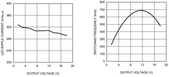
Figure 2. Ripple Current vs. Output Voltage
