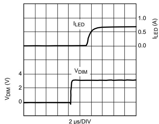
**Figure 6. 1kHz 50% PWM DIMMING (Rising Edge)**
