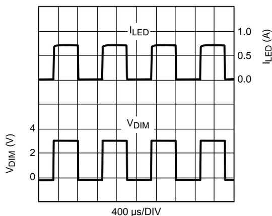
**Figure 5. 1kHz 50% PWM DIMMING**
