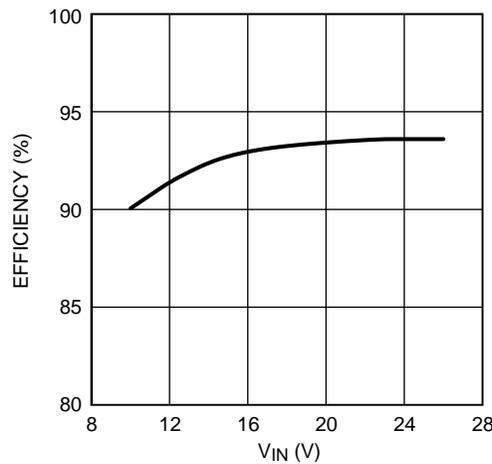
**Figure 1. Efficiency with 9 Series LEDs AT 700mA**
