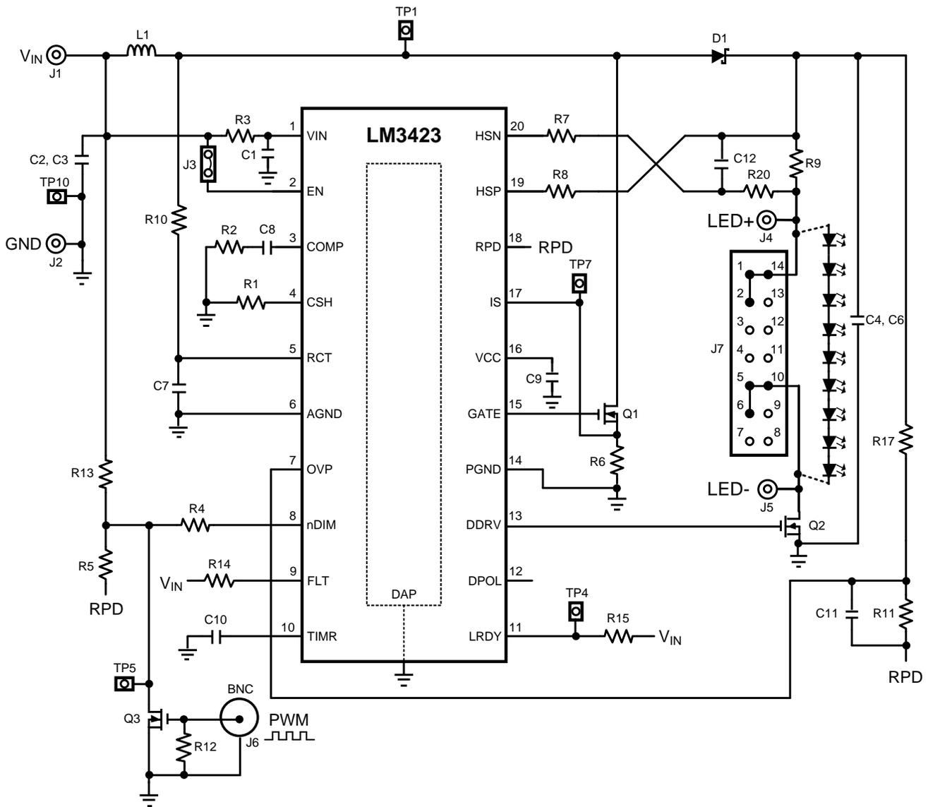
Figure 2. Board Schematic
