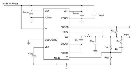
Figure 1-3. LM62440-Q1 Example Application Circuit
