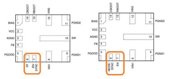
Figure 1-1. LM61440-Q1 Pinout (Left) and LM62440-Q1 Pinout (Right)
