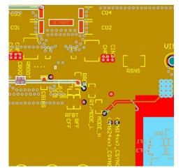
Figure 2-4. Universal PCB Layout Mid Layer 1
