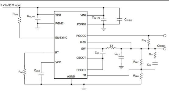
Figure 1-2. LM61440-Q1 Example Application Circuit
