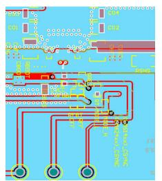
Figure 2-5. Universal PCB Layout Mid Layer 2
